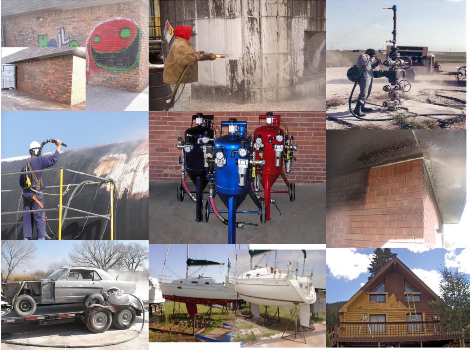
*SurfaceTek's Multi-Media Blaster (MMB)* is a versatile, turn-key system that can utilize a wide range of blast media including: sodium bicarbonate, Super K (potassium sulfate), crushed glass, crushed corn cob, garnet and other abrasives. The *SurfaceTek MMB* system can be used for a wide range of applications: mold remediation, fire & smoke damage restoration, general maintenance, cleaning, degreasing, coating removal and surface preparation.
